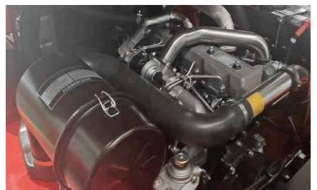
A brand new air filter with a safety filter element makes the engine air intake cleaner and more powerful.
