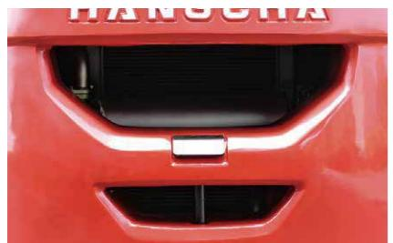
By optimizing the heat dissipation system, the counterweight heat dissipation channel is improved, the air resistance of the heat dissipater is reduced, the cooling efficiency is improved, and the reliable operation of the engine is ensured.
